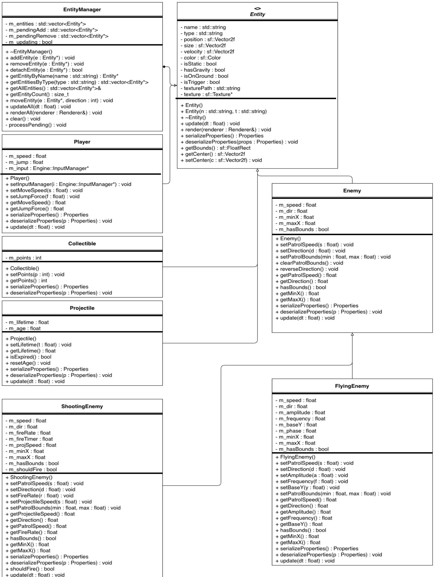
Figure 6: UML Class Diagram of the Entity Subsystem. Illustrating the inheritance hierarchy of game entities and their relationship with the EntityManager.
